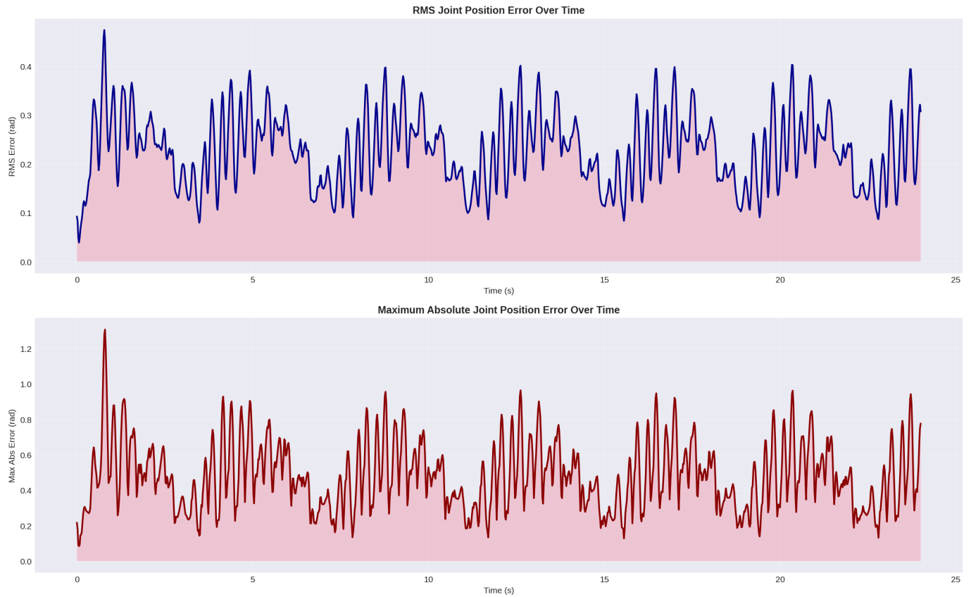
Fig. 5. RMS (top) and Max Absolute (bottom) errors for joint positions over 25 seconds of simulation. The RMS errors represents overall joint position disagreement between the two simulators at each moment in time. The periodic pattern tracks with the gait cycle. It is likely that the peaks are occurring when the leg swing occurs because there's less contact, and thus less constraint. The valleys, where the error is minimized, are likely due to the stanced phase where the robots feet are planted and thus more constrained. For the bottom plot of maximum absolute errors, we see the worst case error at different moments in time. Both forms of joint position error appear stable and do not appear to be growing over time.
